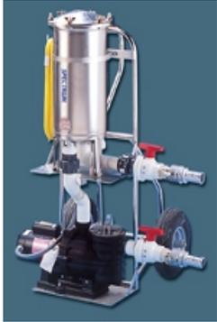
This swimming pool portable vacuum filter uses a 1HP, 110 VAC, Sta-Rite Dyna-Max pump to move approximately 5400 gallons of water per hour through a 155 square foot Harmsco stainless steel cartridge filter. Also available as gas powered if an outlet is not available.
